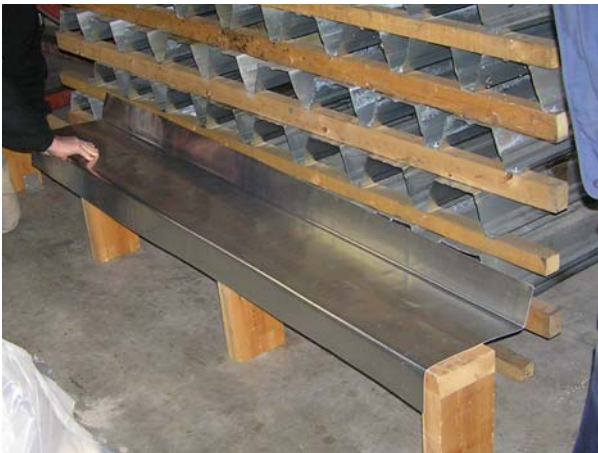
Cutting to size Lengths max. 3-4 metres.
